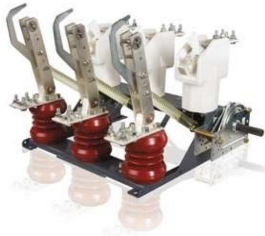
Fig. 23 VersaRupter switch disconnecter VR15 (61 kA)
